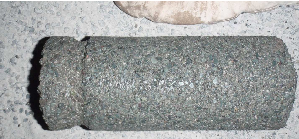
Photo 12: HB12-ND-CORE-DC68-20120307 was drilled around the centerline at station 1+31. Note that the top of the core is augmented in shape as this core was stopped short when the power on the light plant went out. A different light plant was sourced but the top portion of the core remained in glycol (as there was no way to draw it out) while another light plant was rigged up.
